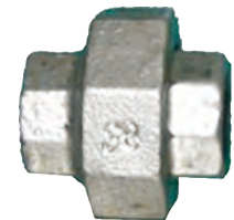
340# union, conical joint, brass to iron seat
